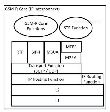
Figure 3: Lower layer protocols and network functions, as seen from IP Interconnect interfaces
