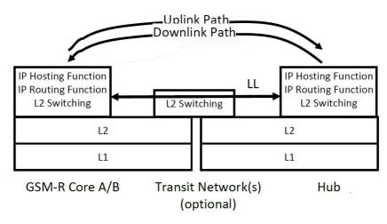
Figure 4: UL/DL IP path, when being switched at transit
