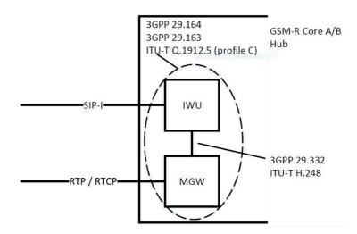
Figure 10: Major Standards for the handling of SIP-I and RTP/RTCP traffic at the edge of the network
